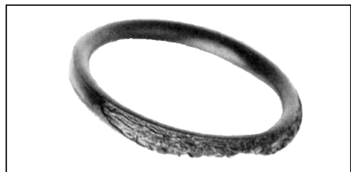
Figure 10-3: "Nibbled" Extruded O-Ring
